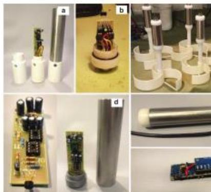
Fig. 5: General view of the conductivity sensor (a), wind speed sensor (b, c), suspended solids sensor (d), and wave sensor (e).
